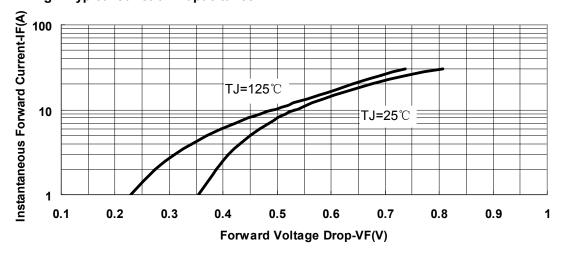
Fig.3-Typical Forward Voltage Drop Characteristics
